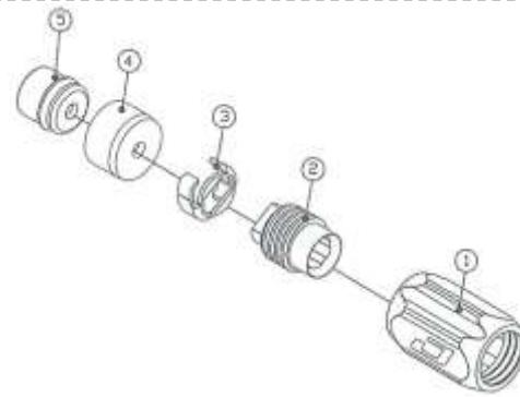
**Integrated mechanical cable stop:**
