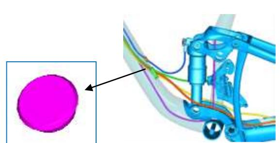
**HT Cable Guide L Side for Front/Rear Derailleur Cable**
