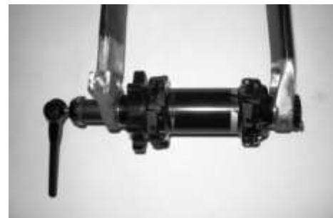
Step 1: Fasten lock nut onto dropout at right fork leg to hand tight.
