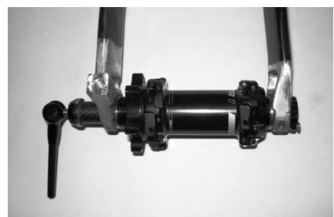
Step 1: Fasten lock nut onto dropout at right fork leg to hand tight.
