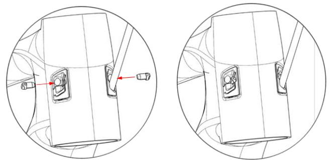
**Step 5 : Installing the Guide PE Tube for the R.D.**
